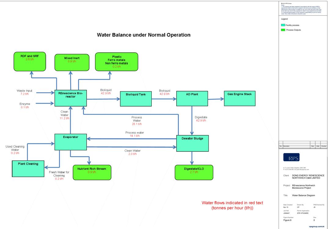
Q2:515 RPS scoop Vision 1. This drawing has been prepared in accordance with the scope of RPS's appointment with a licent and is subject to the terms and conditions of that appointment. RPS accepts no slability for any use of this document ofter than by its dient and only for the purposes for which was prepared and provided. 2. If received electronically is the necipient's responsibility to print to cornect scalas. Christ withme dimensions should be used.
