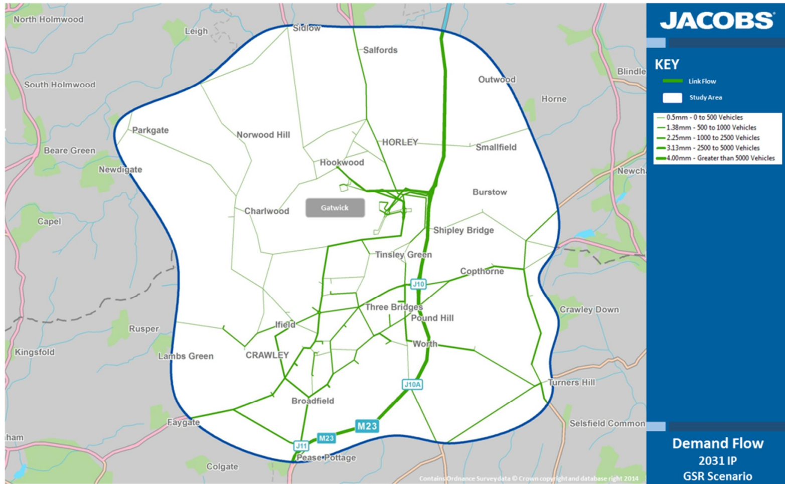
Figure 5: Demand Traffic Flows Gatwick Second Runway IP on the local road network within the immediate vicinity of Gatwick
