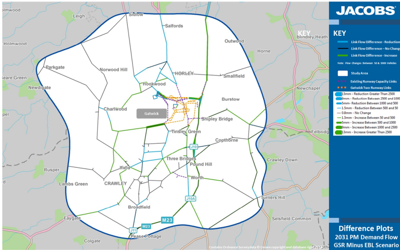
Figure 9: Demand Traffic Flows Difference PM on the local road network within the immediate vicinity of Gatwick
