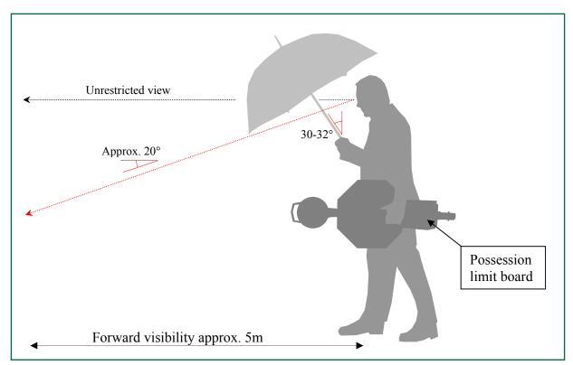
Figure 8: Diagram showing effect of 10 mph wind on forward sighting when using an umbrella
