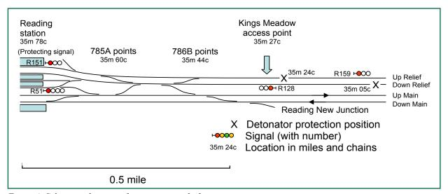
Figure 4: Schematic diagram of site prior to end of possession
