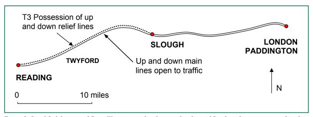
Figure 2: Simplified diagram of Great Western main line between London and Reading showing section of track under possession
