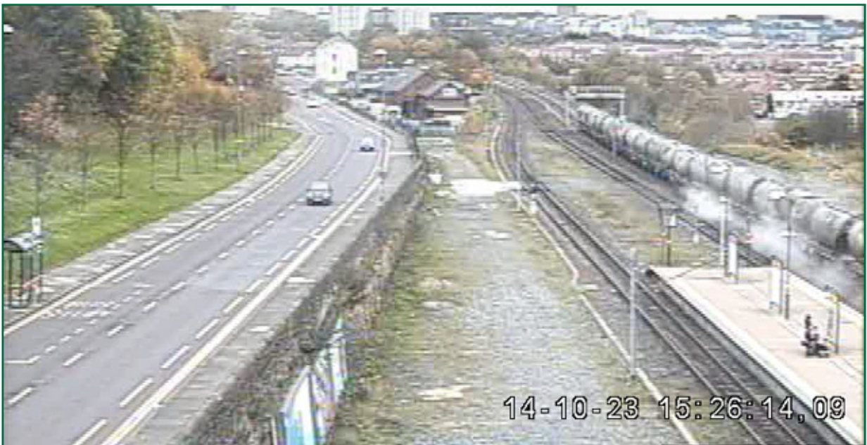
Figure 6: CCTV image of the derailed wagon passing Felling Metro station (image courtesy of DB Regio Tyne and Wear Metro)
