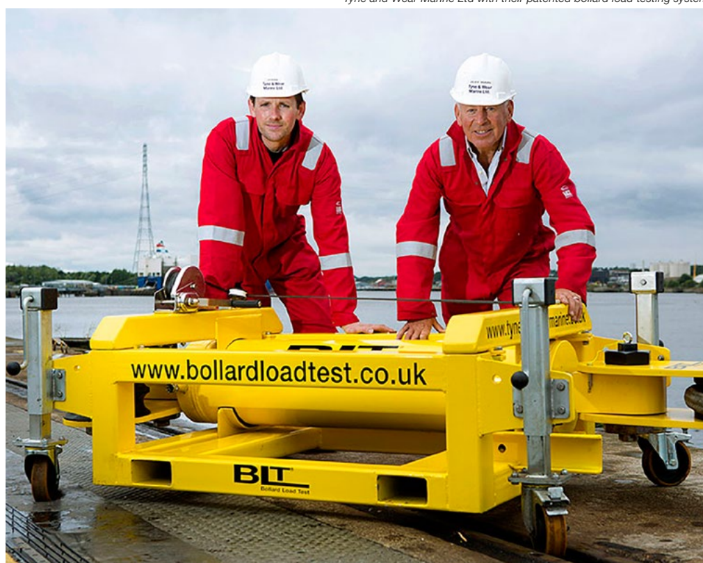
Tyne and Wear Marine Ltd with their patented bollard load testing system
