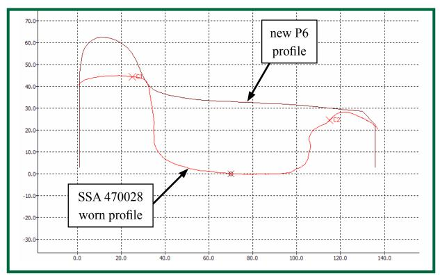
Figure 17: Profile of right leading wheel near centre of large flat
