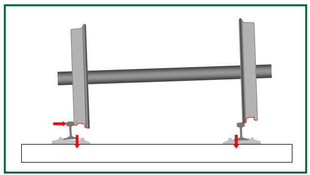
Figure 10: 35 sleepers after the point of derailment. As right wheel passes adjustment switches, it is catapulted into free flight. Resistance to gauge spreading forces exerted by the left rail caused the wheelset to be displaced sideways leading to full derailment to the right.
