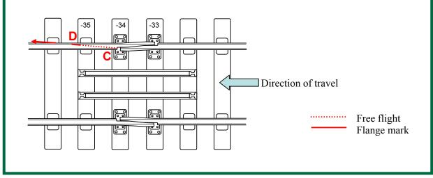
*Figure 9: Full derailment triggered by impact of right wheel with machined notch in adjustment switch layout* (**C**). *Flange landed on rail head after free flight of approx 700 mm at* (**D**). *Sleeper numbers are indicated. Figure 11 uses the same notation.*
