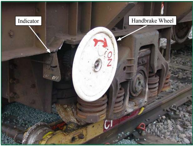
Figure 13: Handbrake wheel and indicator on SSA 470028
