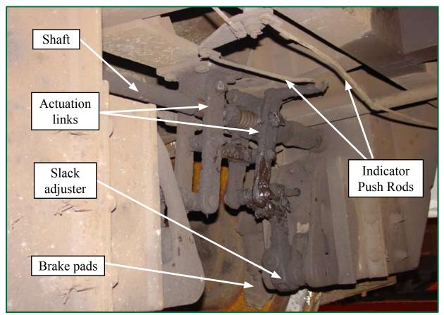
Figure 14: SSA 470028 handbrake components below the underframe.
