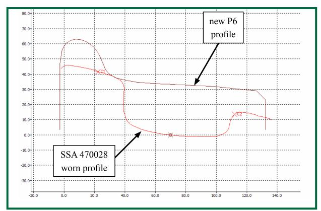
Figure 16: Profile of left leading wheel near centre of large flat
