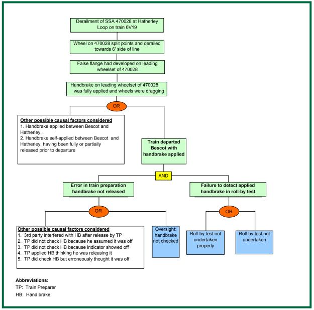
Figure 21: Causal analysis diagram
