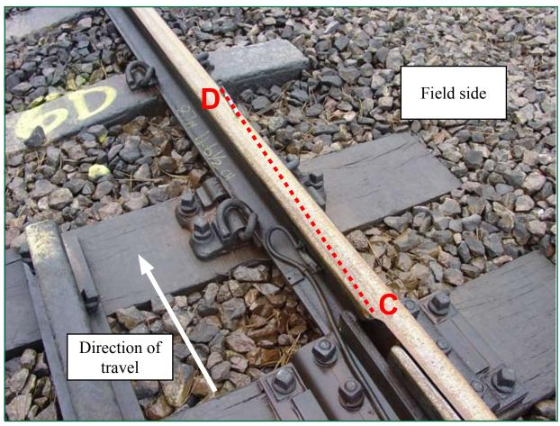
Figure 11: Photograph of adjustment switches showing point of impact with the machined notch (C) and derailment mark indicated by the position of the pen on rail head (D) where right hand wheel landed after being in free flight for 700 mm (grinding marks are visible on the rail head, showing light corrosion following overnight rain).
