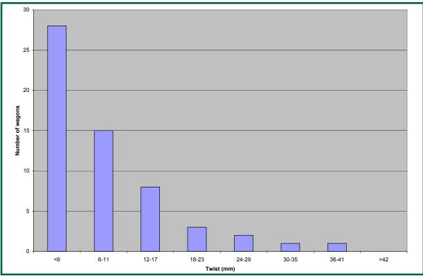
Figure 8: Results of the wagon frame twist survey
