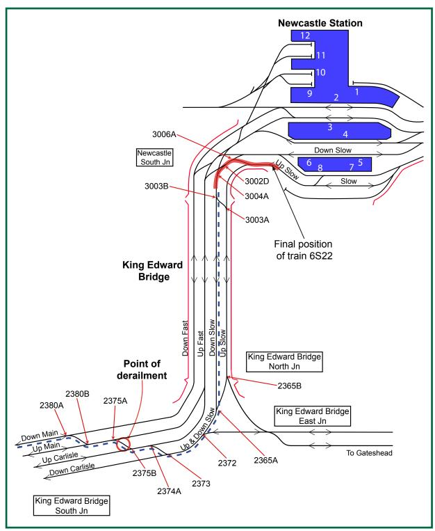
Figure 2: Schematic track diagram in the vicinity of the derailment
