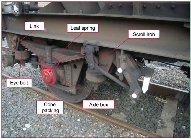
Figure 4: An HAA suspension arrangement
