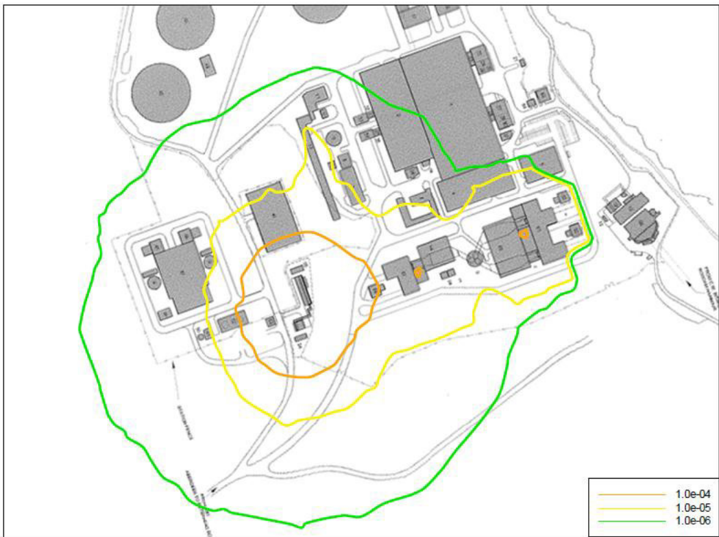
Contours showing the frequency of flame impingement regardless of duration
