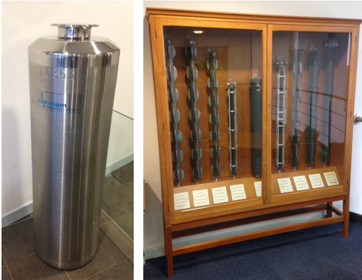
Figure 8 - Example container for vitrified High Level Waste (HLW) (left) and fuel rods for nuclear reactors (right).
