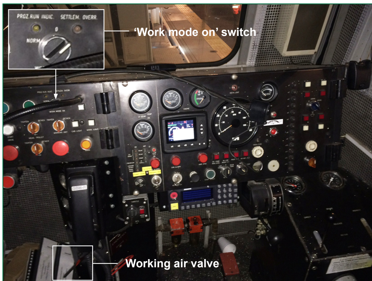
Figure 11: Photograph of the working cab taken at 02:54 hrs by the RAIB's accredited agent
