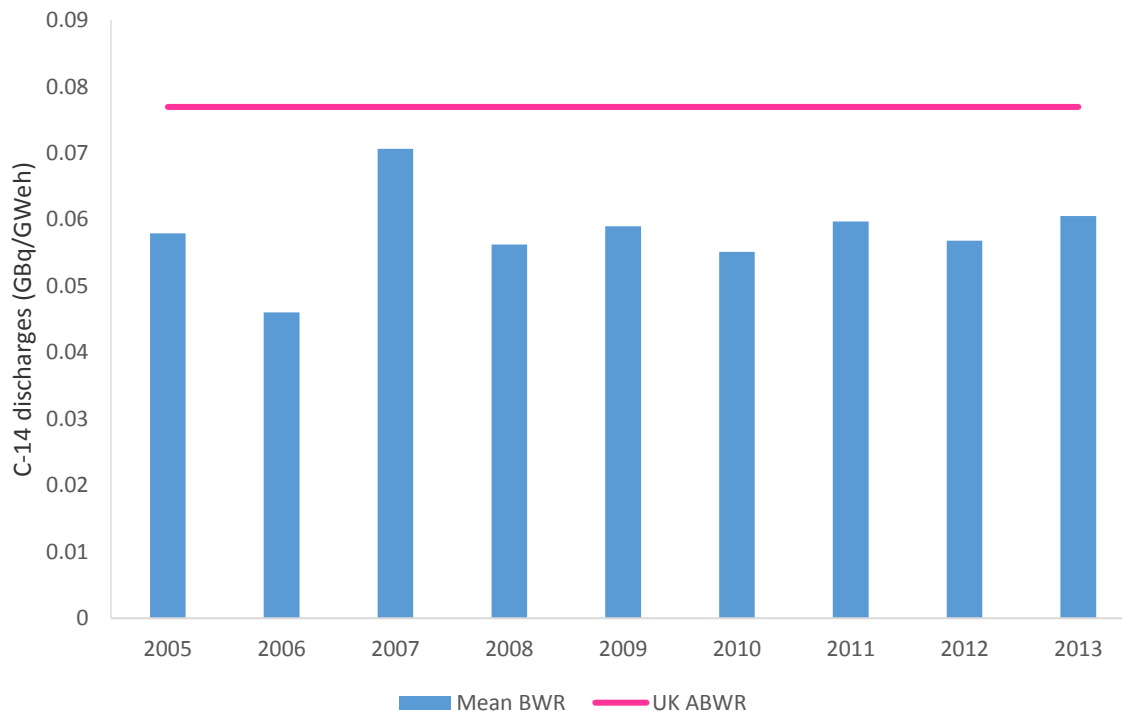
Figure 5: Mean normalised annual gaseous carbon-14 discharges from BWRs 2005 to 2013 Pink line shows normalised UK ABWR estimated annual gaseous carbon-14 discharges
