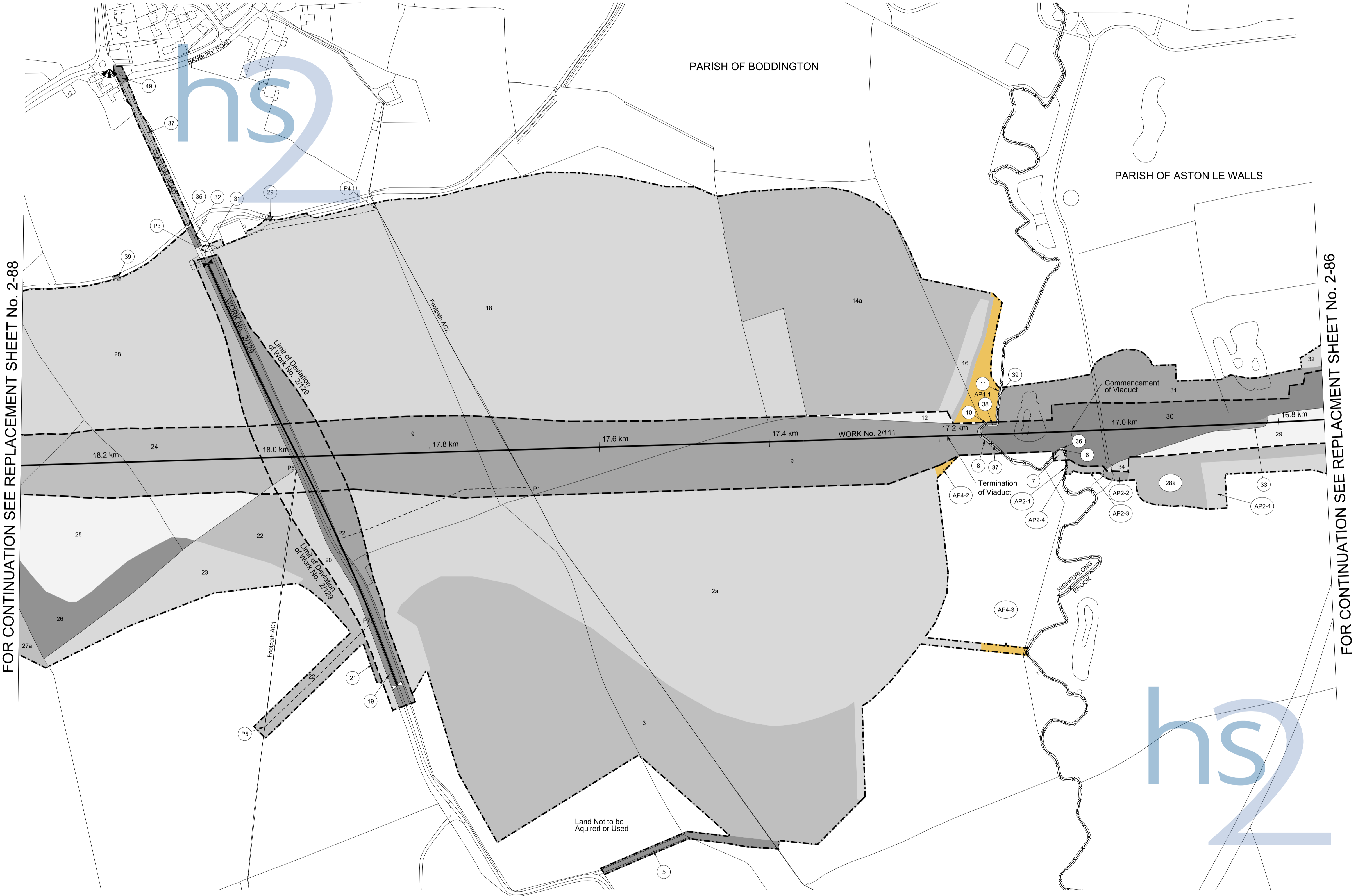
Proposed Viaduct over Highfurlong Brook Work No. 2/111 Span 20.0m, Headway 4.10m
