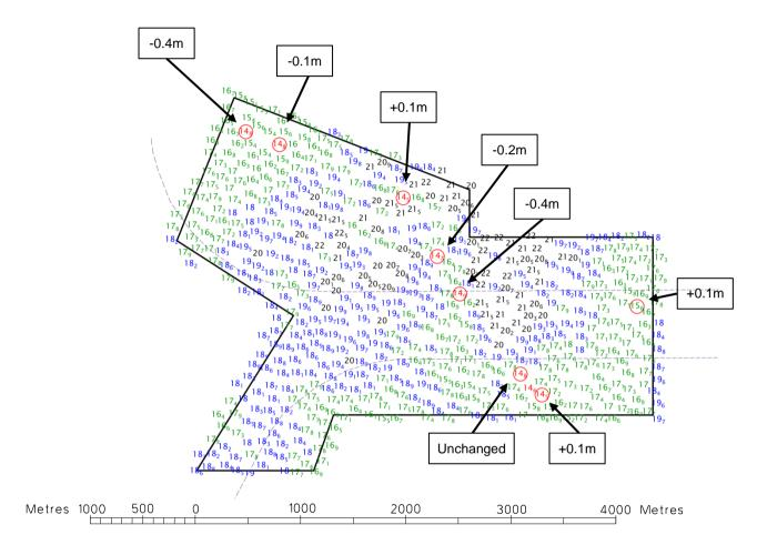
Depth changes indicated above are from the closest corresponding 2014 sounding available. Hence depth differences will be from different positions from the 2015 sounding selection as an automatic shoal bias sounding selection tool has been utilised which produces a representation of the shoal values in a data set.
