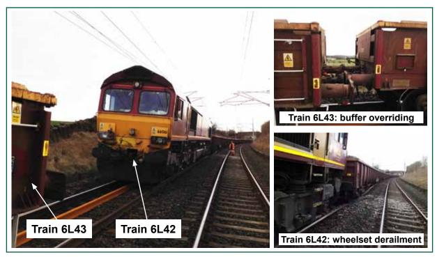
Figure 2: Trains 6L43 and 6L42 after the collision (photographs courtesy of Network Rail)
