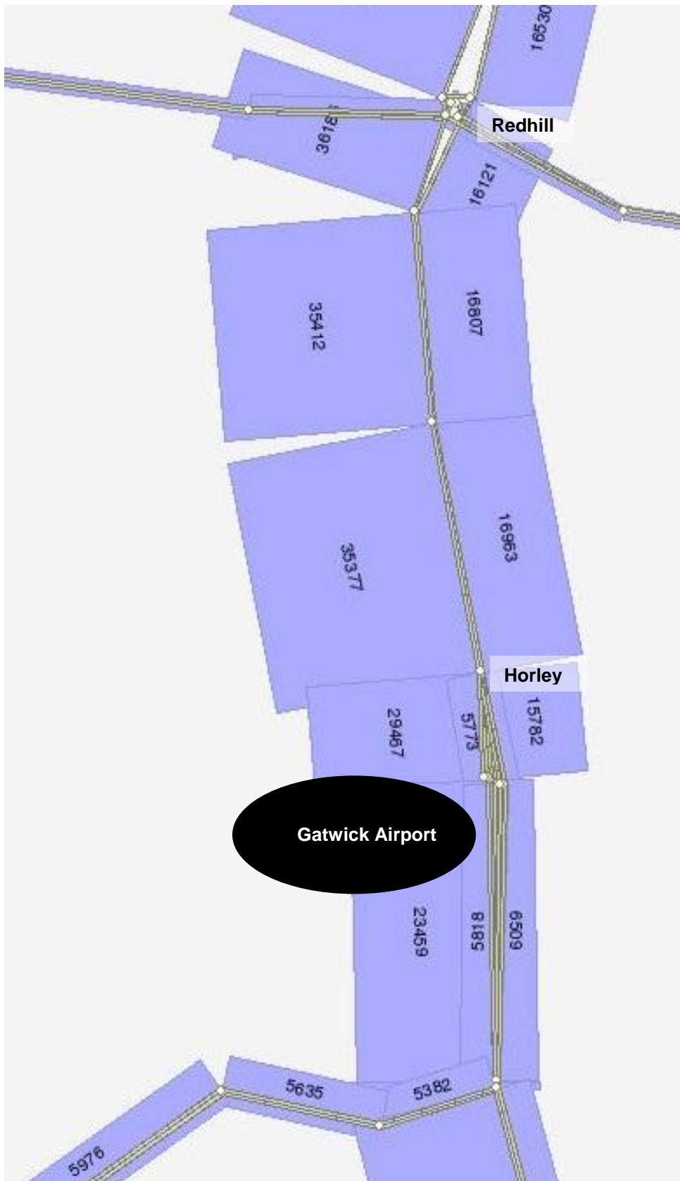
Figure 4-23: 2031 Extended Baseline AM peak forecast rail demand around Gatwick (with Second Runway)
