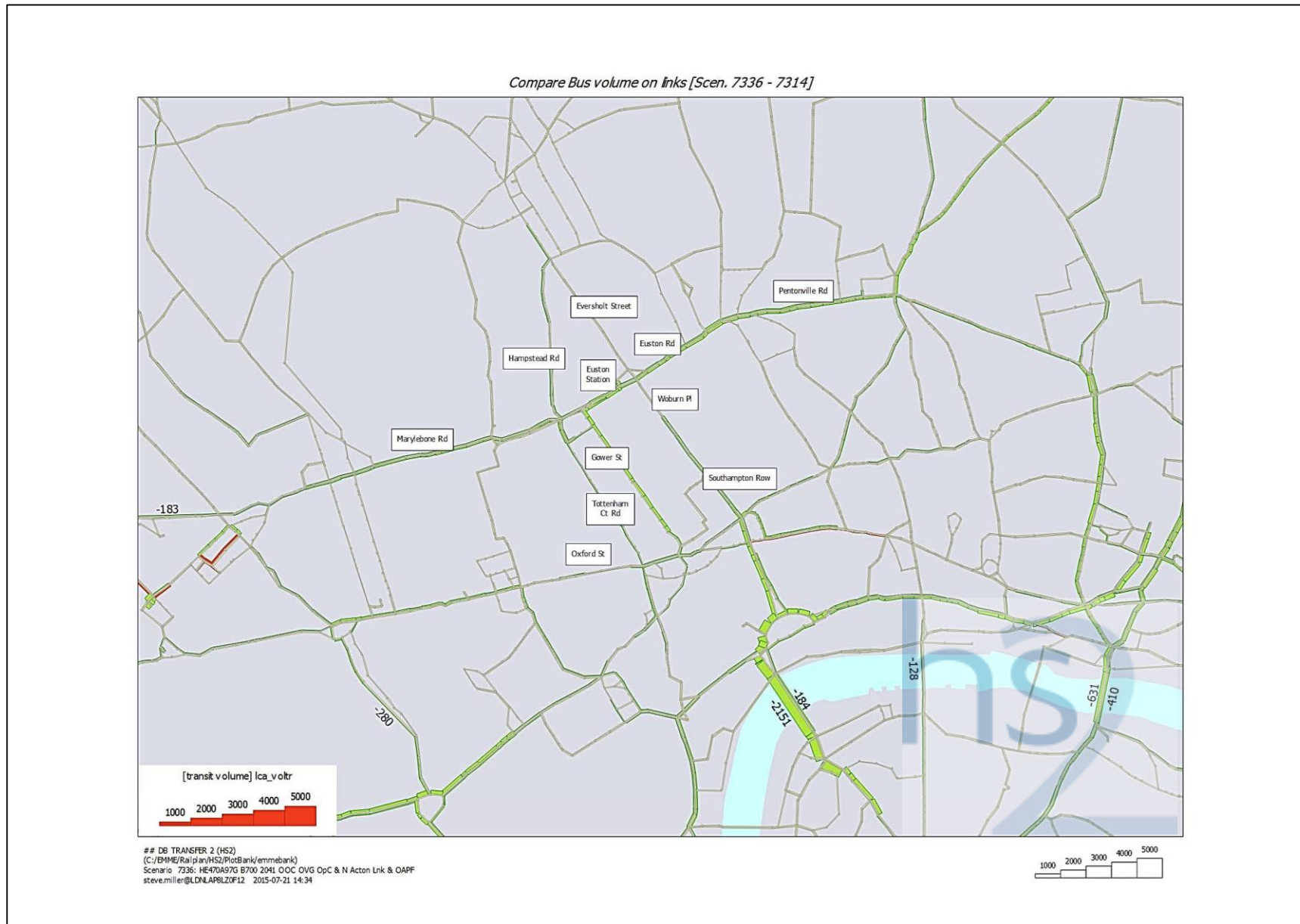
Figure 219: Bus flow differences 2041 AM peak Overground at Old Oak Common station with OAPF
