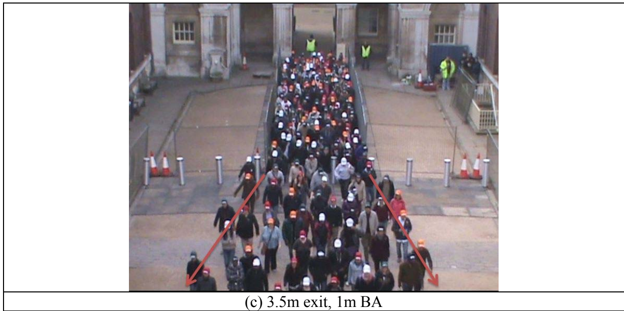
Figure 71:TS3 – Diffusion in the exiting crowd for the (a) NoBA with 4.5m exit, (b) 1m BA with 4.5m exit and (c) 1m BA with 3.5m exit.
