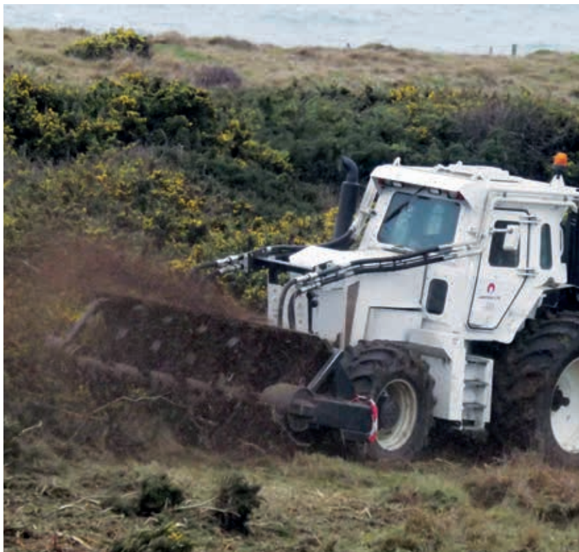
The Armtrac 100-350, a formidable piece of equipment that can spin seventy chains at 800rpm © A. Cheeseman
