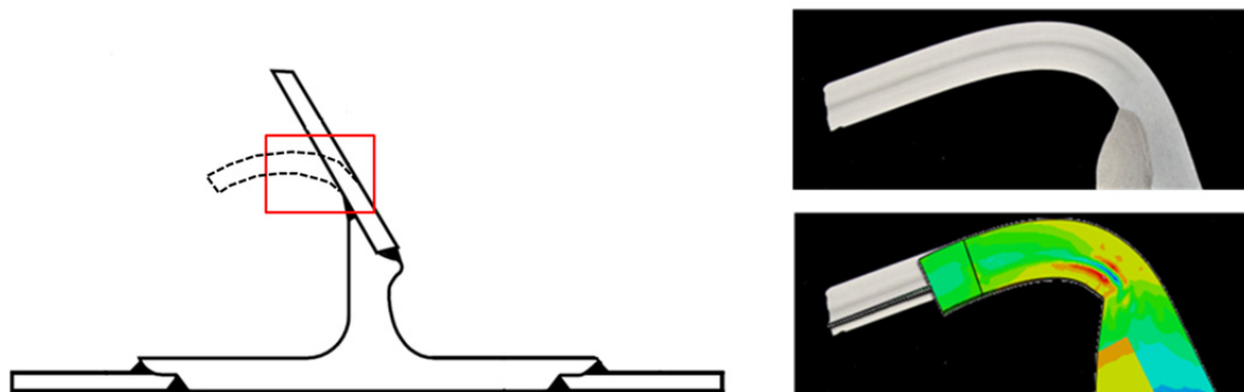
Figure 26 FEA results superimposed on the macro-section AT11-1475-RO-05 taken from the centre of the crush zone (equivalent to the symmetry plane in the FE model). Deformation not magnified, and equivalent plastic strain contour shown for reference.
