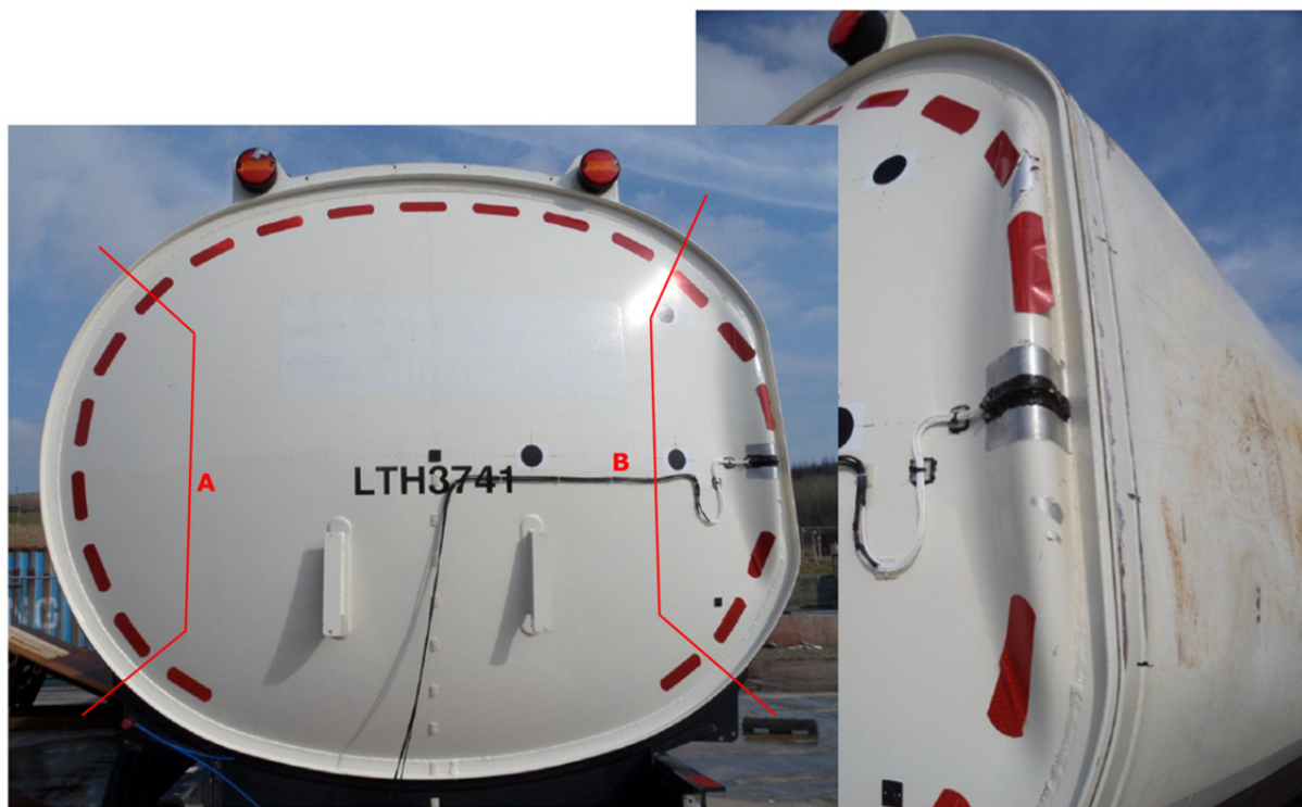
Figure 2 Locations of the sections removed from the impacted, rear offside of AT11-1475 (Position B) and the undamaged, rear nearside (Position A). Images provided courtesy of HSL.
