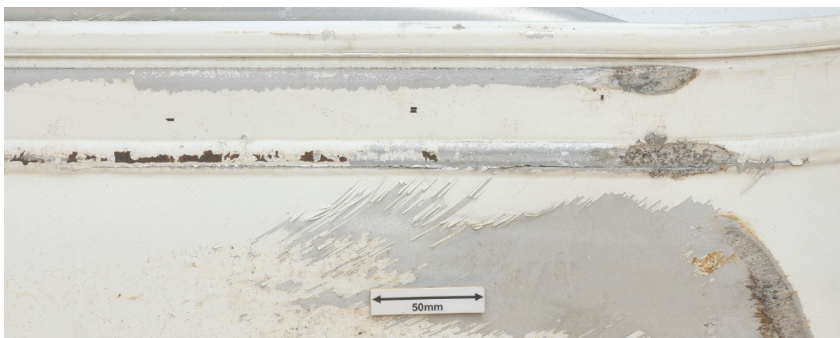
Figure J3 J2580 Band H O/S sample longitudinal crack.
