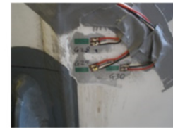
Figure B5 Illustration of the positions of strain gauges G28-37 for band D/10(+).
