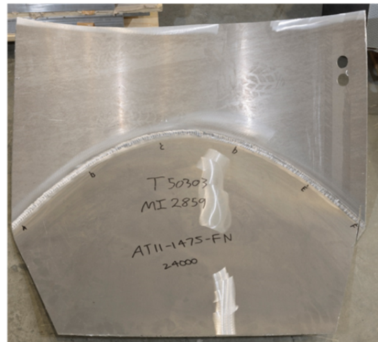
Figure 18 Diagram of the sampling plan for the front nearside (undamaged) section of AT11-1475.
