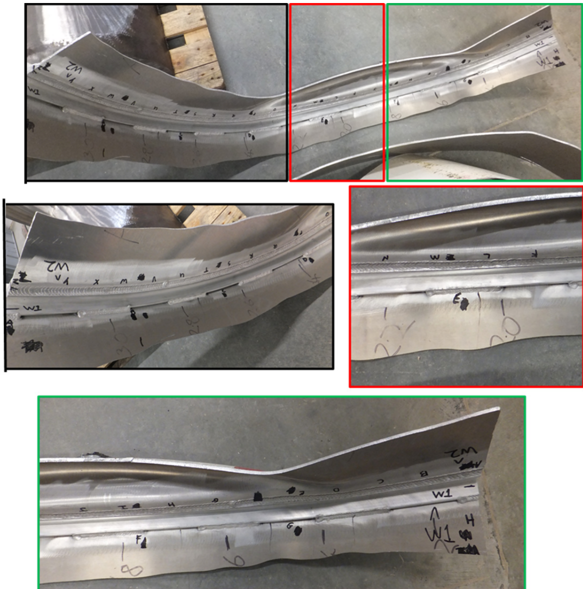
Figure 4 Image of the section from the rear offside of AT11-1475 showing the datum markers (A-H for the primary circumferential weld) for the radiographic examination (see Table 1).
