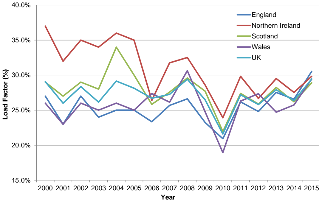
Chart 14: Onshore wind load factor on an unchanged configuration basis, by UK country
