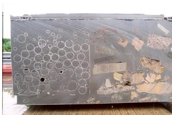
A cross-section of a grouted waste container, courtesy of LLW Repository Ltd.
