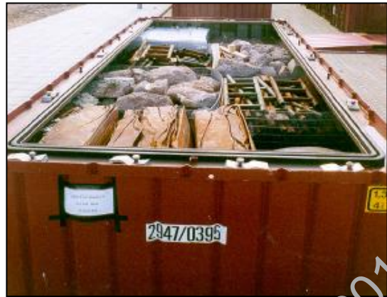
Typical ISO container of waste prior to grouting, courtesy of LLW Repository Ltd
