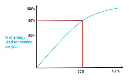
Heat pump size as a % of total capacity of the heating system
