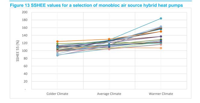
The average SSHEE at 55°C for air to water heat pumps at average climate conditions was 119% and the maximum and minimum 133% and 108% respectively. The SSHEE value gives the performance in primary energy terms and converting these to performance in terms of delivered electricity by multiplying by 2.5/100 implies approximate seasonal performance factors (SPF) ranging from 2.6 to 3.75 which are all greater than the minimum SPF of 2.5 required for renewable energy.
