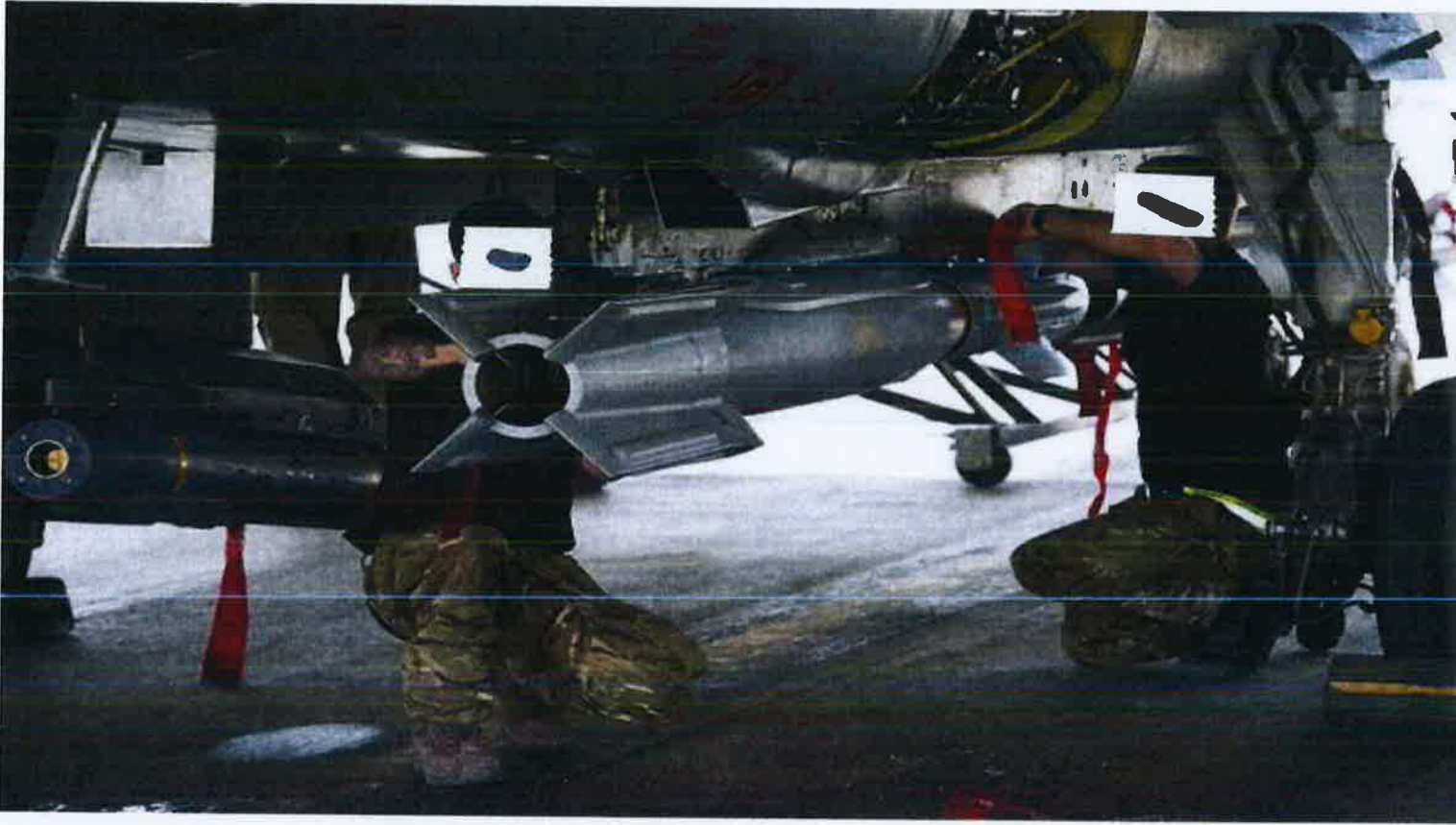
Figure 3-4-9. EAW Personnel Fitting Paveway IV Bomb to GR4 Tornado
