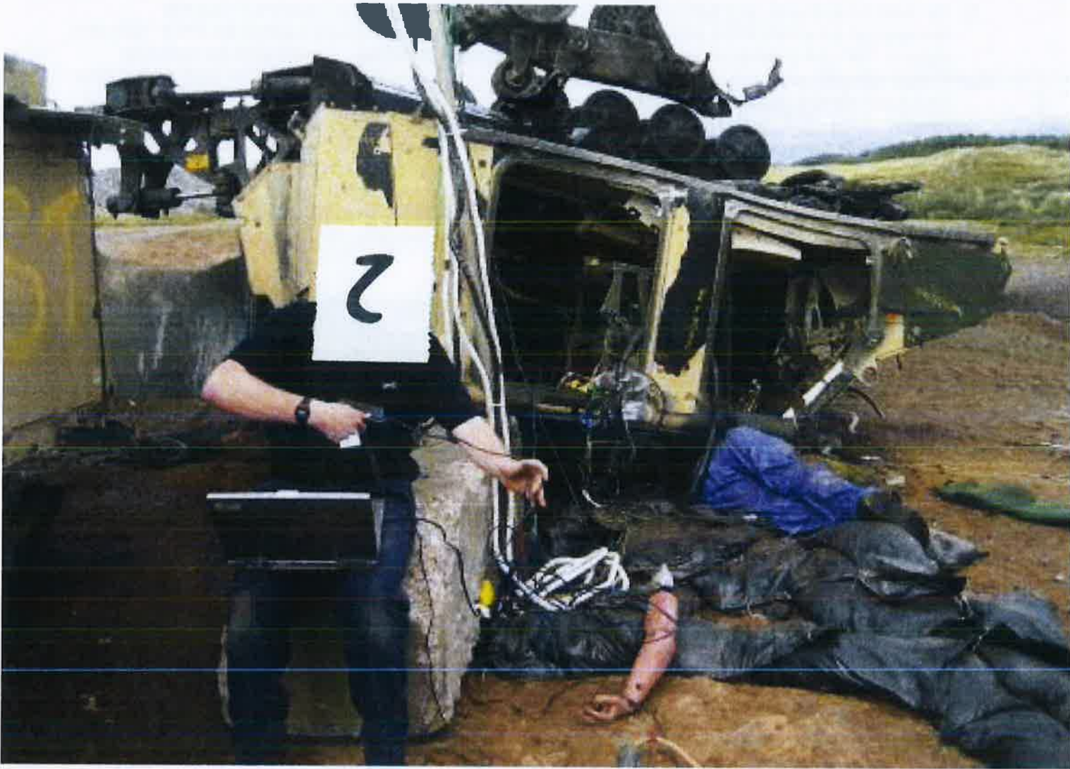
Fig 1-3-7 Seat belt testing in response to theatre reach back
