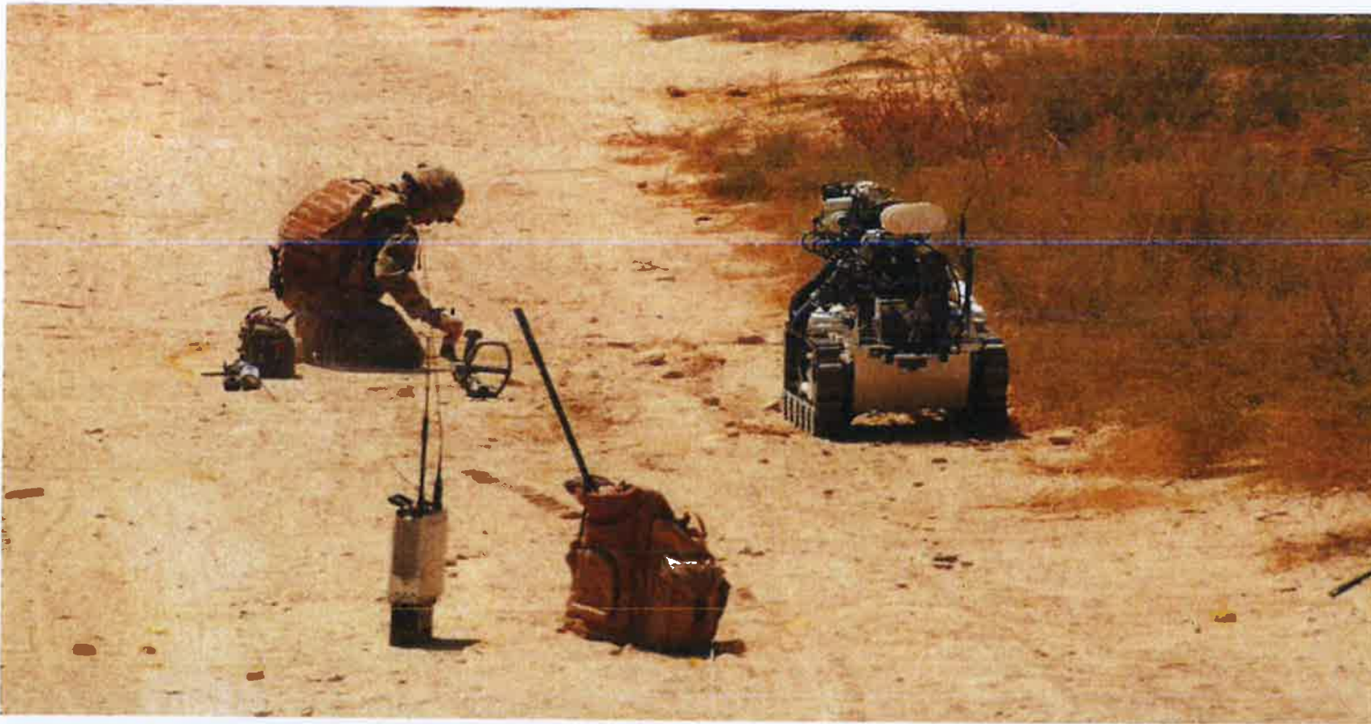
Figure 3-6-10 IEDD operator confirming an IED using manual techniques with RCV in support.
