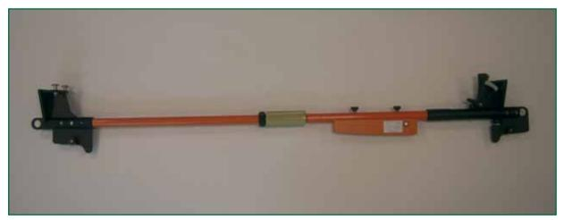
*Figure 9: A TGP8 gauge (not the one used at 201A points) - note the dummy wheel profiles on lower left and right extremities.*
