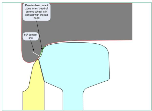
Figure 14: Diagram showing how the TGP8 gauge was used on 31 August 2007 (not to scale)
