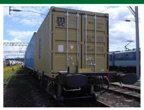
Marks Tey: Container flat wagon (type FSA/FTA) derailed on a series of dips in the track. Wagon type did not meet vertical ride performance requirements in standards when partially loaded.
