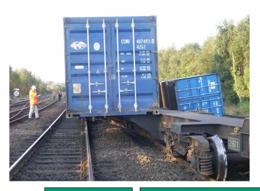
Duddeston: Leading wheelset derailed due wheel unloading. Load on wagon resulted in combination of lateral and longitudinal asymmetry
