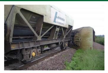
Ely Dock Junction and Wigan: Wagons had frame twist with incorrect packing that worsened the amount of twist.
