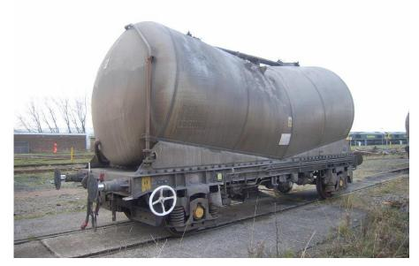
Heworth: Leading left hand wheel derailed due to an un-damped Gloucester pedestal suspension on leading right hand wheel. Worn components were found within this suspension. Recommendation to mitigate risk of degraded ride performance due to worn suspension components.
