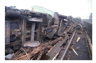
Bordesley Junction: Trailing left hand suspension locked-up causing leading right hand wheel to unload and flange climb.
