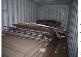
Sheet steel inside container was offset to left-hand side
