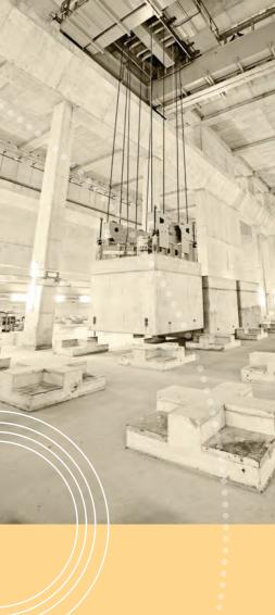
Top right - ILW being moved into storage at the interim waste store at Trawsfynydd pending ultimate disposal. Bottom left - On the Vitrification Store charge floor. Ensuring the safety of the most hazardous waste on the NDA estate.
