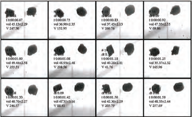
Figure 3 Multiple stream of pellets of deuterium ice in-flight launched from the improved JET High Frequency Pellet Injector system
