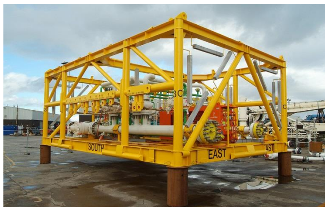
Atlantic Manifold Piping Skid (fits inside protection structure)
