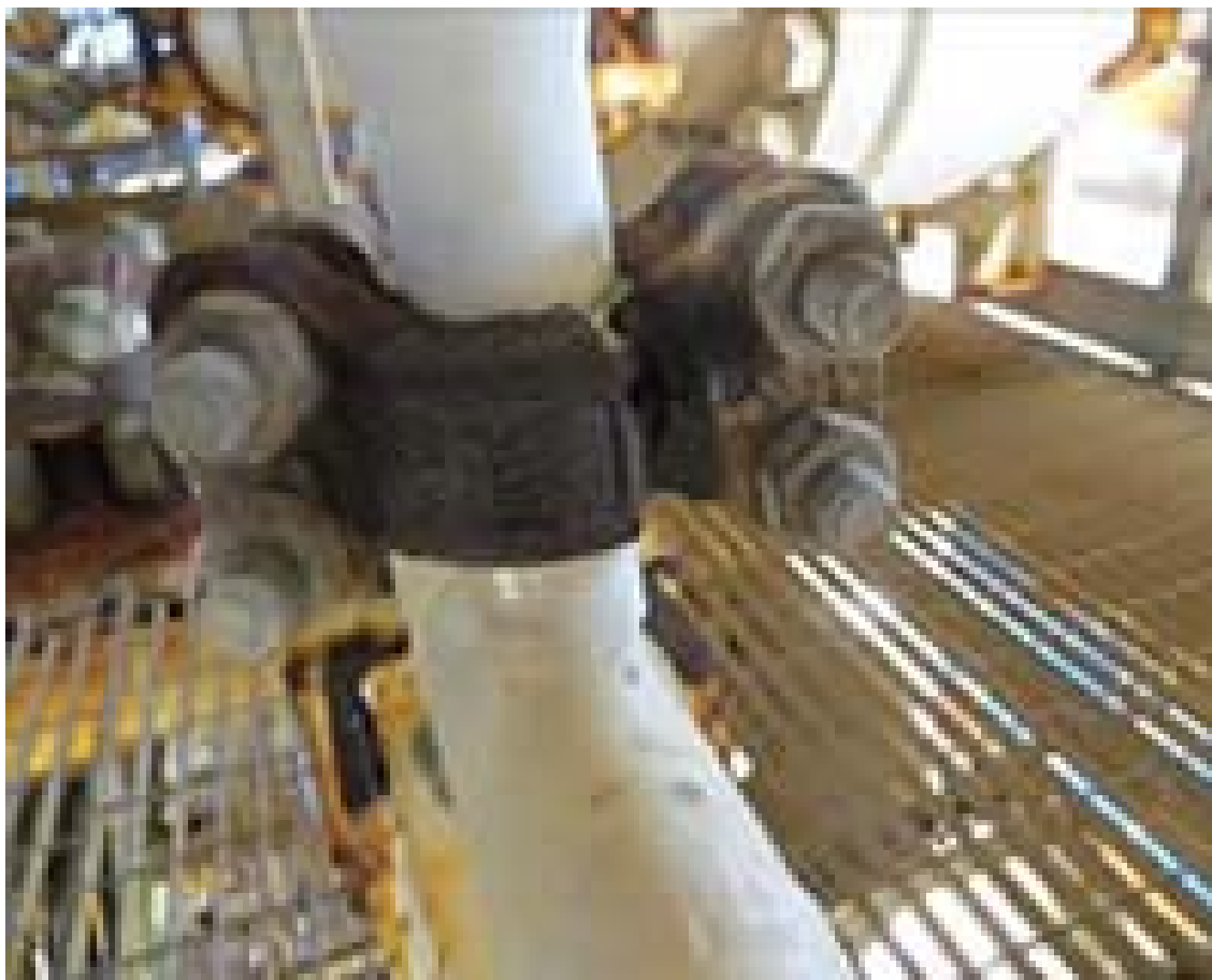
Figure 1 Showing Cracking caused by poor heat treatment during manufacturing process
