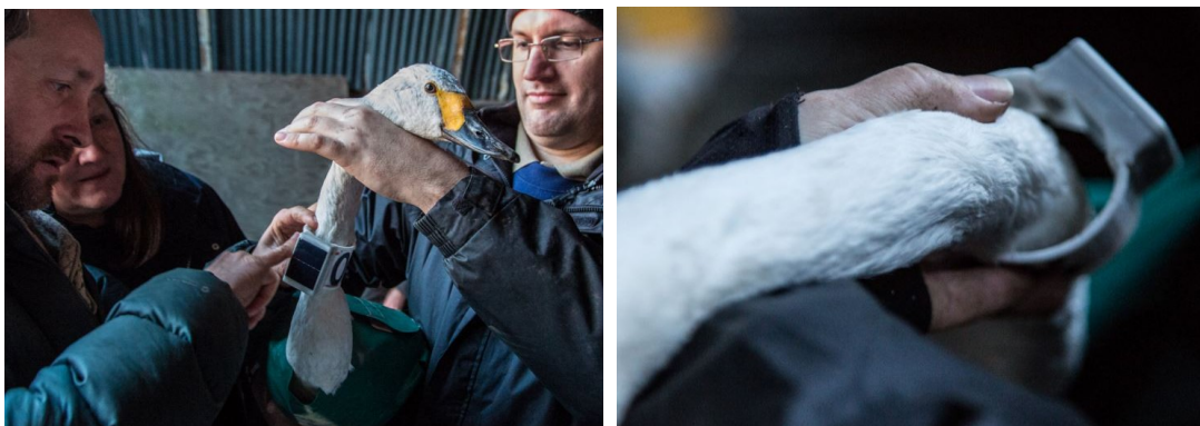
Figure 1. Fitting the solar Ecotone UHF-GSM-GPS collar-mounted device to a Bewick's Swan and the gap between the swan's neck and the device once fitted.
