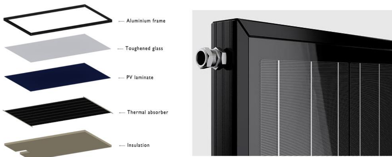
Figure 7 Example of a type 2 unglazed PV-T module with insulation (Solar Angel, 2015)
