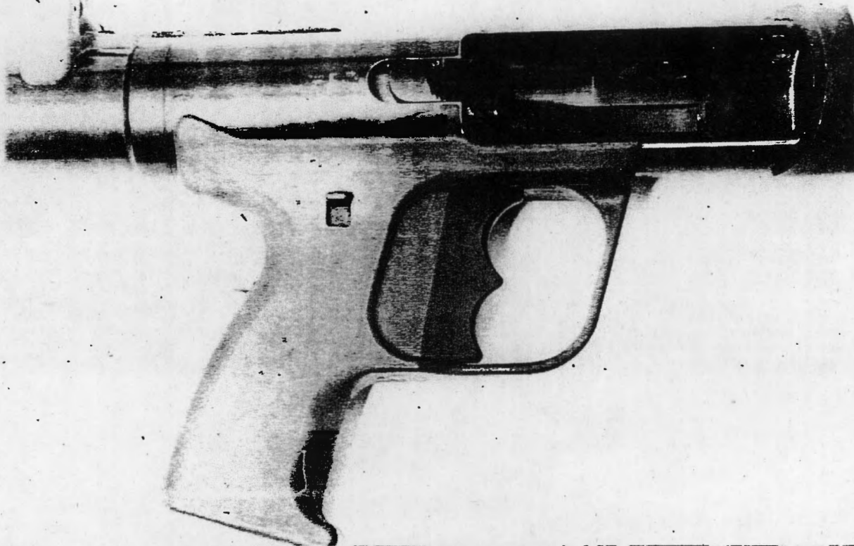
Fig 7. Pistol Grip Showing the 2 Safety Catches.
