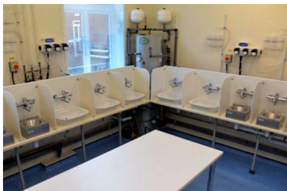
PHE laboratory sink and drain model for the investigation of control measures for CPE in hospitals
