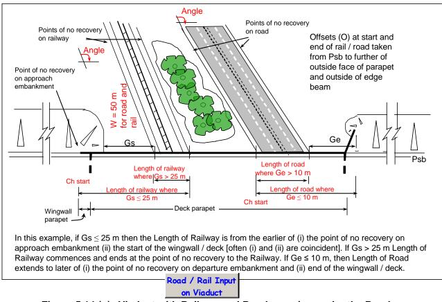
Figure 5.14 (g) Viaduct with Railway and Road crossing under the Road
