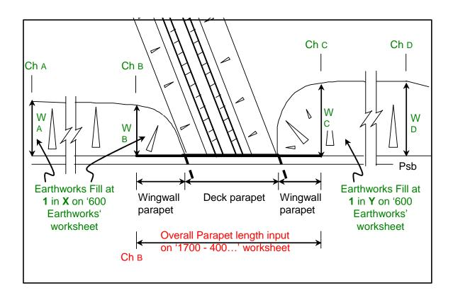
The following figures identify how information relating to Parapets and to Earthworks are input into the respective worksheets.
