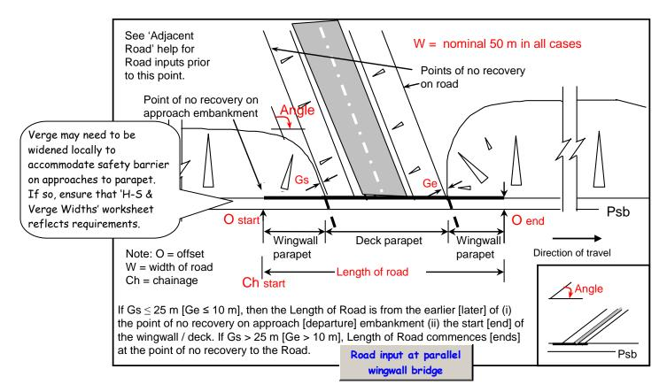
Figure 5.15 (e) Road crossing under Road at structure with parallel wingwalls
