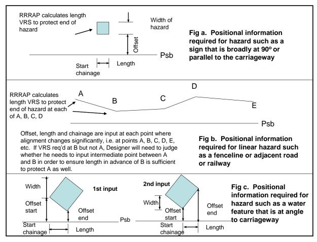
Fig 1-4 Positional information required by RRRAP in order to calculate VRS requirements – note that this gives typical details; further particulars are contained within each of the relevant sections.
