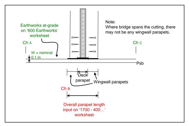
Figure 5.9 (c) - Parapet and Earthworks Inputs at Underbridge when road at-grade
