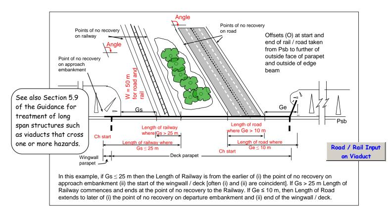
Figure 5.15 (d) Viaduct with Road and Railway crossing under the Road
