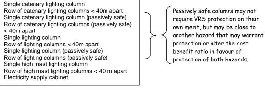
**5.6.1** High Masts. A high mast is one that exceeds 18m in height.
