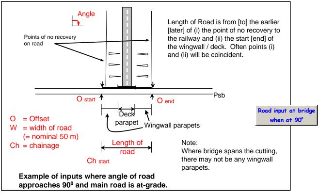
Figure 5.15 (g) Road crossing under Road where at-grade and or at 90°
