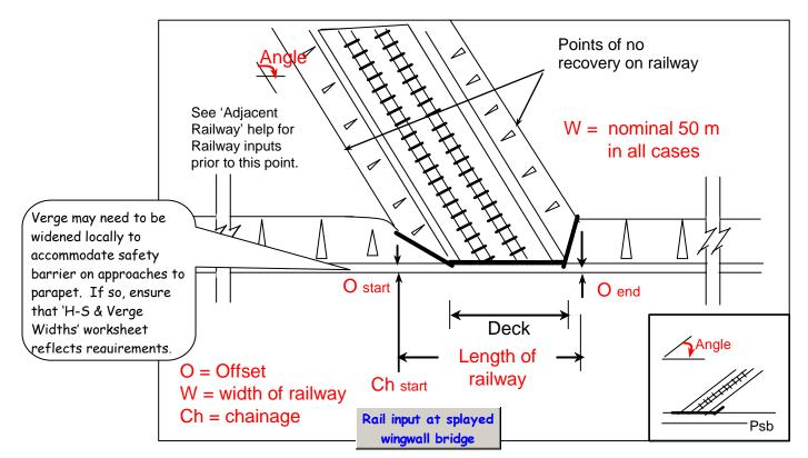
Figure 5.14 (e) Railway crossing under Road at structure with splayed wingwalls
