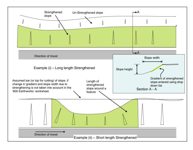
Figure 5.10 (a) Strengthened Slopes
