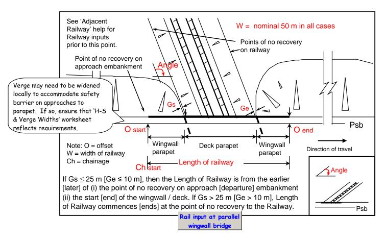
Figure 5.14 (d) Railway crossing under Road at structure with parallel wingwalls
