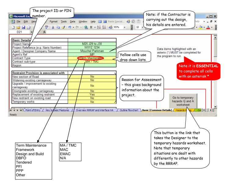
**3.3** Details Relating to Particular Section Covered by Assessment. The middle part of the spreadsheet, shown below, is used to record details of the particular Section of the road that is under consideration. A road that has a length of Slip Road and a length of Mainline will need to be split into two Sections, as the traffic flows and cross section, alignment and hence run-off and accident characteristics of the Slip and Mainline will be different.
