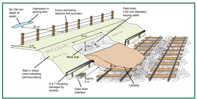
Figure 7: Cutting slope after landslip
