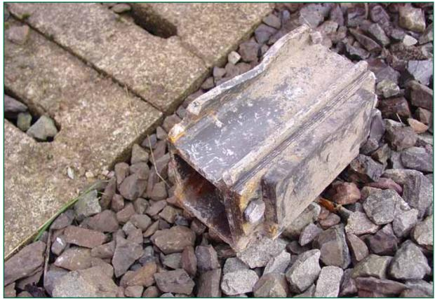
Figure 11: Coupler lateral bump stop in the 'as found' condition
