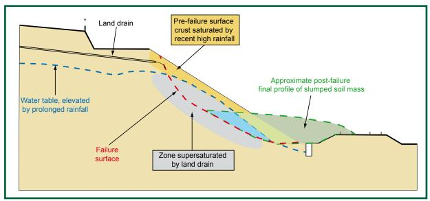
Figure 10: Sketch section through the failed cutting slope
