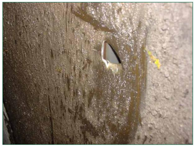
Figure 3: Hole in fuel tank
