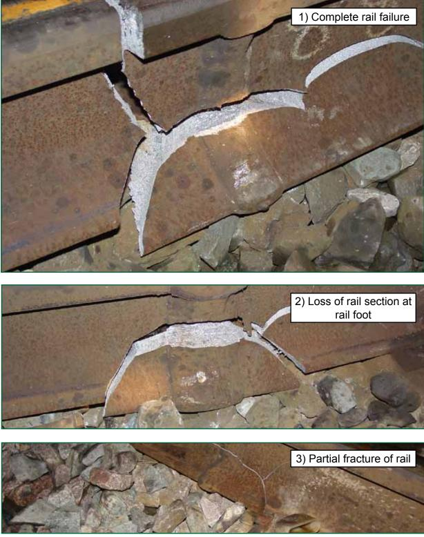
Figure 4: Examples of three different types of rail fractures observed
