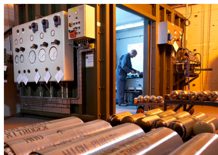
Pictured above; The pressure test cell. Cylinders under test
