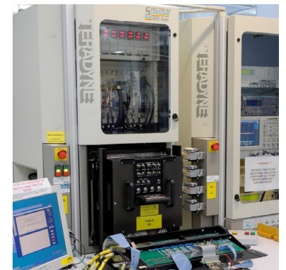
Teradyne automatic test equipment in the DECA Automatic Test Equipment centre of excellence
