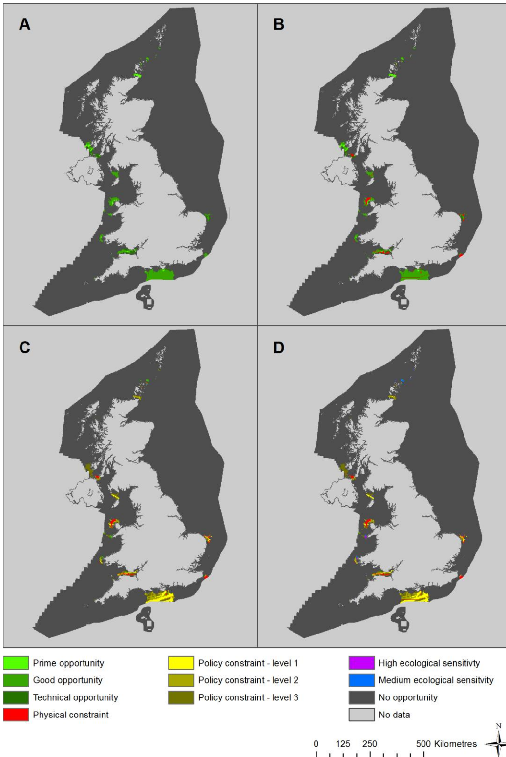
Figure A10. Opportunity and constraint mapping for offshore tidal stream energy. A) Opportunity map for tidal stream developments (light green is prime opportunity, mid-green is good opportunity and dark green is technical opportunity); B) opportunity map for tidal stream developments overlaid with physical constraints (red) to exploiting the resource; C) opportunity map for tidal stream developments overlaid with physical and policy constraints (from level 1, least constrained, in light yellow, to level 3, most constrained, in brown) to exploiting the resource; D) opportunity map for tidal stream developments with physical and policy constraints to exploiting the resource applied, remaining areas of opportunity are overlaid with areas of high (purple) and medium (blue) ecological sensitivity to offshore wind.
