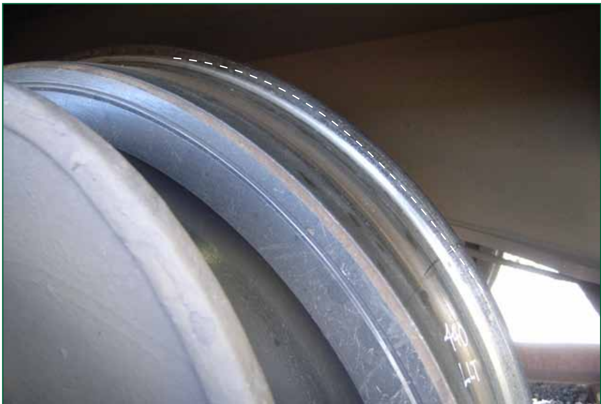
Figure 13: Possible climb marks on the left-hand wheel of the trailing wheelset of the rear bogie of wagon 608440
