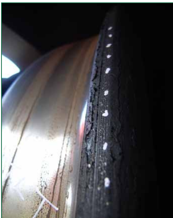
Figure 14: Contact marks on the left-hand wheel of the trailing wheelset of the rear bogie of wagon 607129
