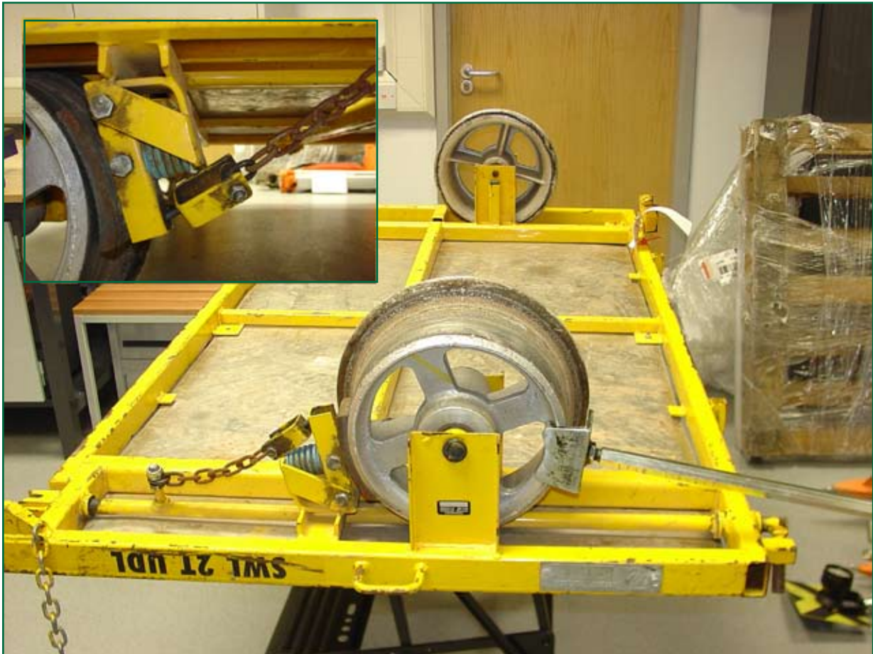
Figure 23: Image showing trolley, brake block and associated linkage (reference trolley)
