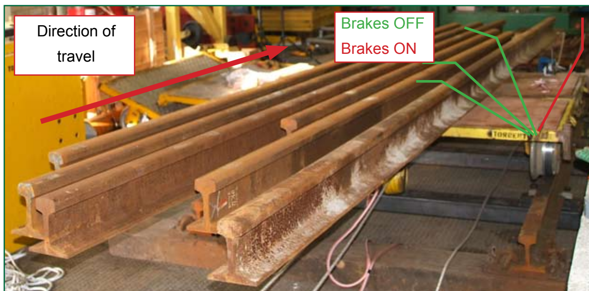
Figure 15: Image of incident trolley RT10574 showing incident rails in position and handle positions
