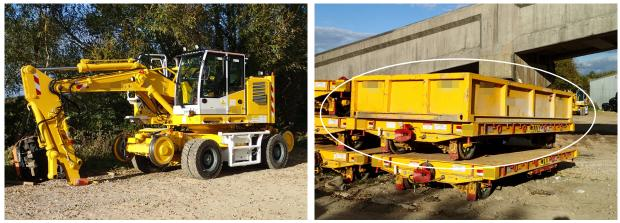
Figure 4: Example of a road/rail machine (left) and trailer and ballast box combination (circled right) similar to that used by the work group but not involved with the incident.
