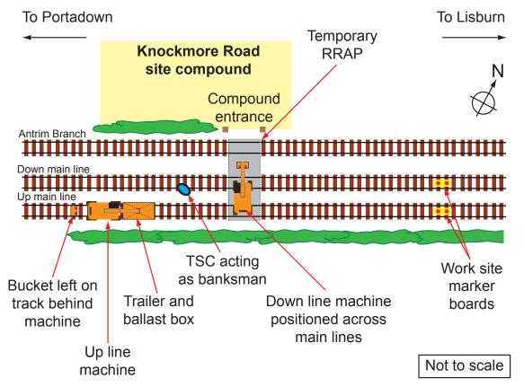
Figure 10: Location of the equipment and the TSC immediately before lifting the trailer and ballast box into the cess
