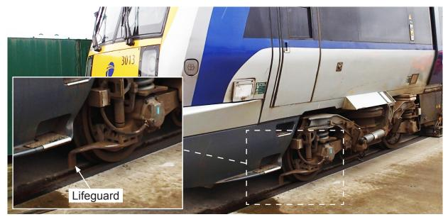
Figure 8: Side view of train B301 after the accident showing the left side lifeguard ahead of the leading bogie
