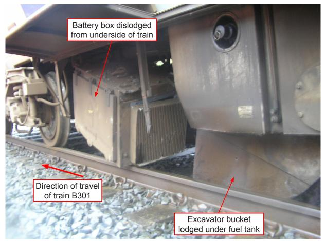
Figure 9: Vehicle damage and excavator bucket under train B301
