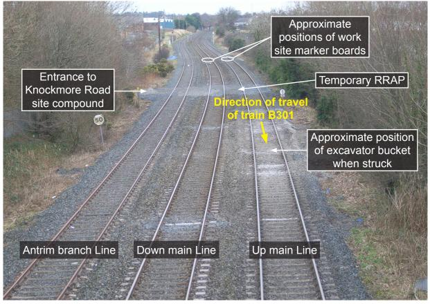
Figure 2: RRAP and worksite marker board location near Knockmore Road site compound
