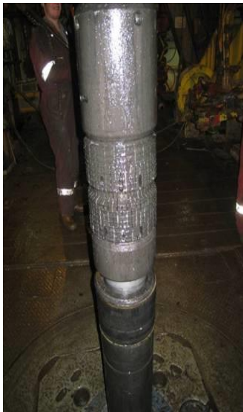
Figure 4-1: HHC Packer at rotary table after being retrieved from well Pierce A10
