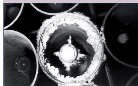
Corroded fuel couldn't be retrieved using conventional methods
