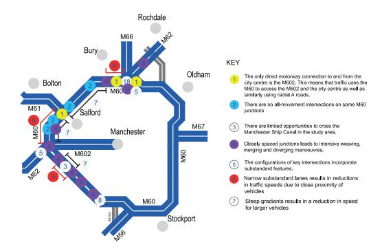
Figure 2 - Existing Motorway Network Alignment & Junction Issues
