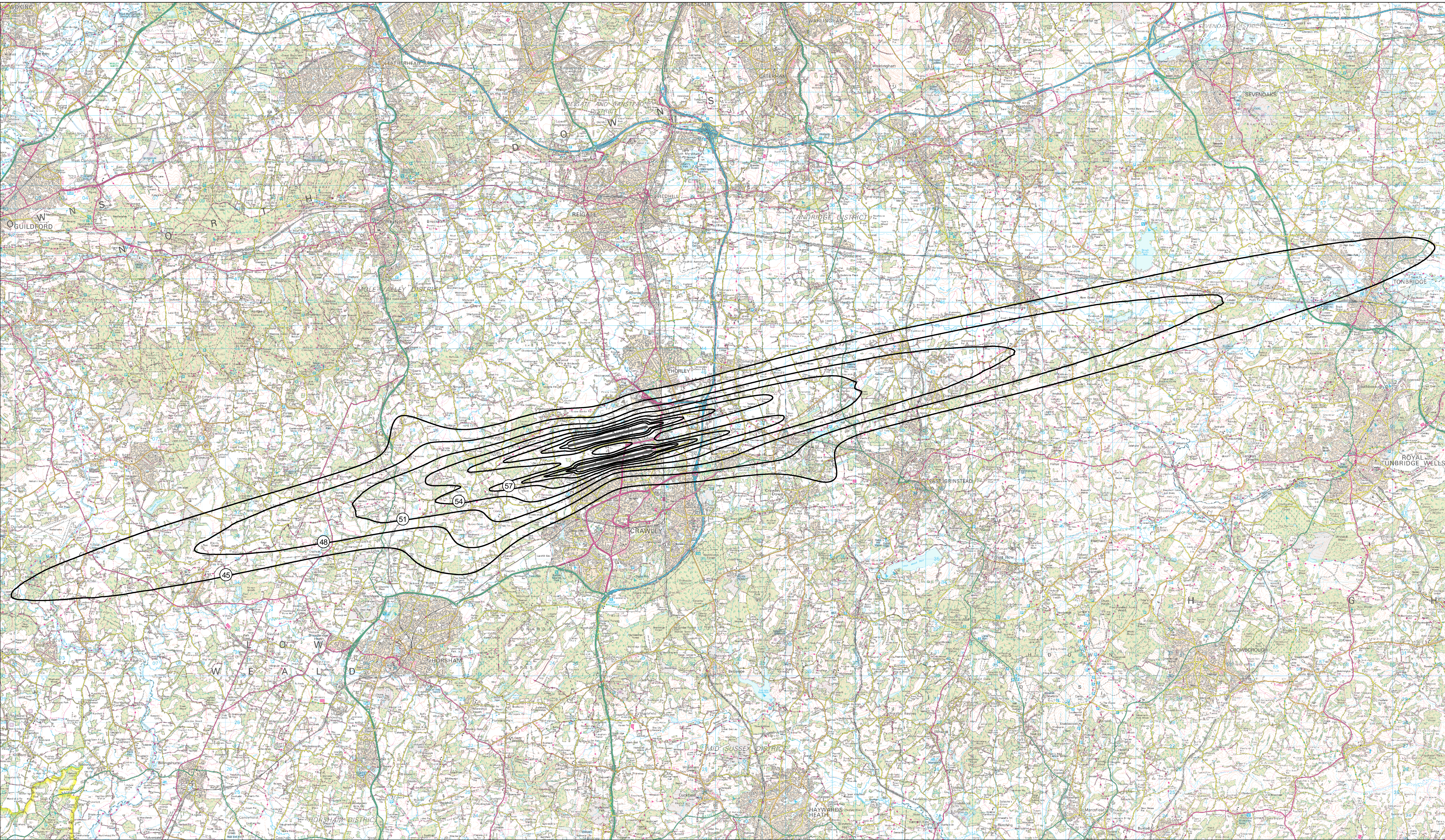
GATWICK AIRPORT 95mppa R2 Option 3 (Wide Spaced Mixed Mode) No EATs 2050 L night 45-66 dB(A) Contours Modal split 68% west / 32% east
