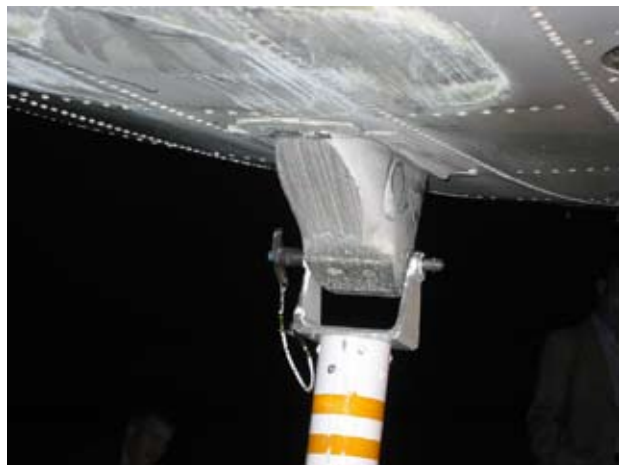
Abrasion damage on fuselage underside
