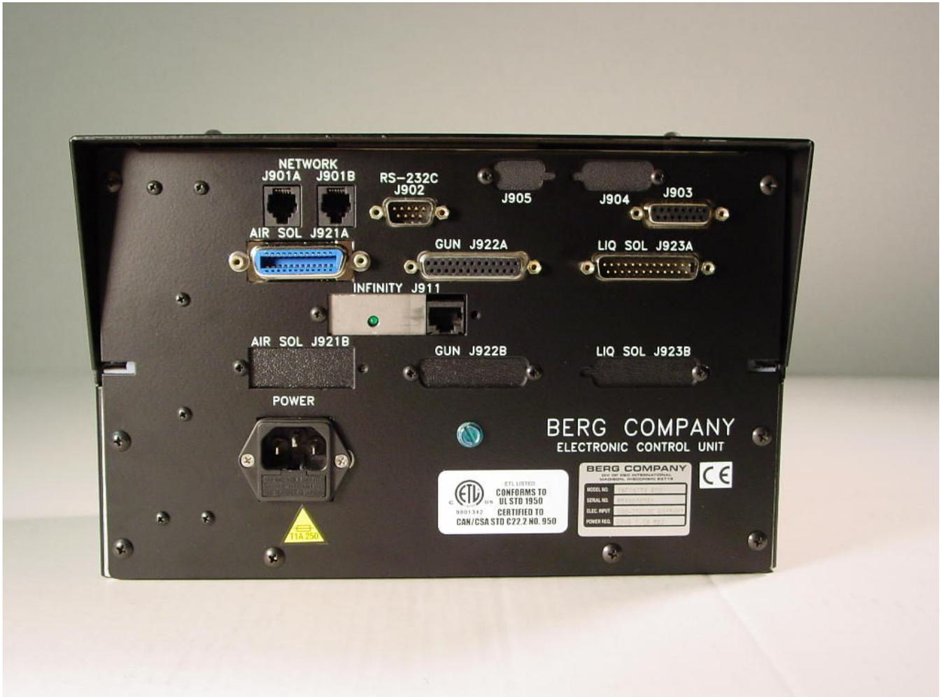
**Figure 7 Infinity Electronic Control Unit (ECU)**
