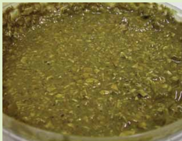
Figure 3: A slurry must be created to help ensure that toxins derived from mould growth are sampled representatively
