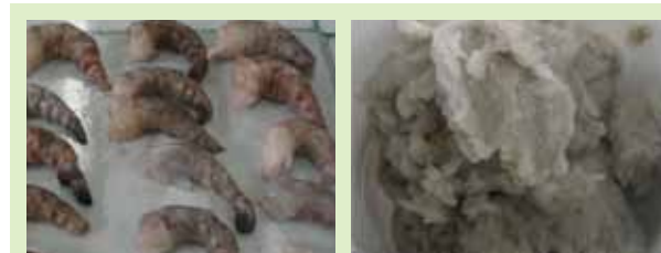
Figure 2: Prawns were coned and quartered, shelled, washed, and finally blended as a prelude to referee analysis for nitrofuran metabolites
