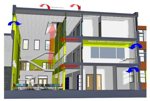
The sports hall has high level actuated windows to allow cross ventilation without excessive air movement within the occupied zone.
