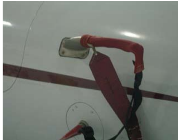
Right pitot probe and AOA vane below Kevlar cover
